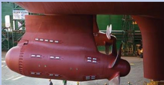
Azipod Propulsion Unit Source: Samsung Heavy Industries
